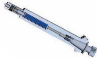
Fig. 4.8: Schematic representation of a tool clamping component
