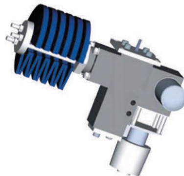
Fig. 4.3: Schematic representation of an energy storage system with springs
