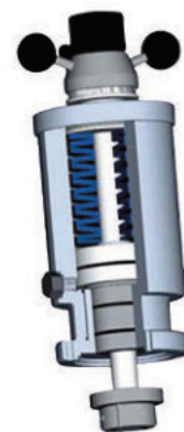
Fig. 4.6: Schematic representation of a piston return assembly
