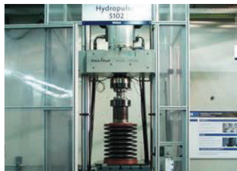
Fig. 6.2: Life time test of disc spring stacks
